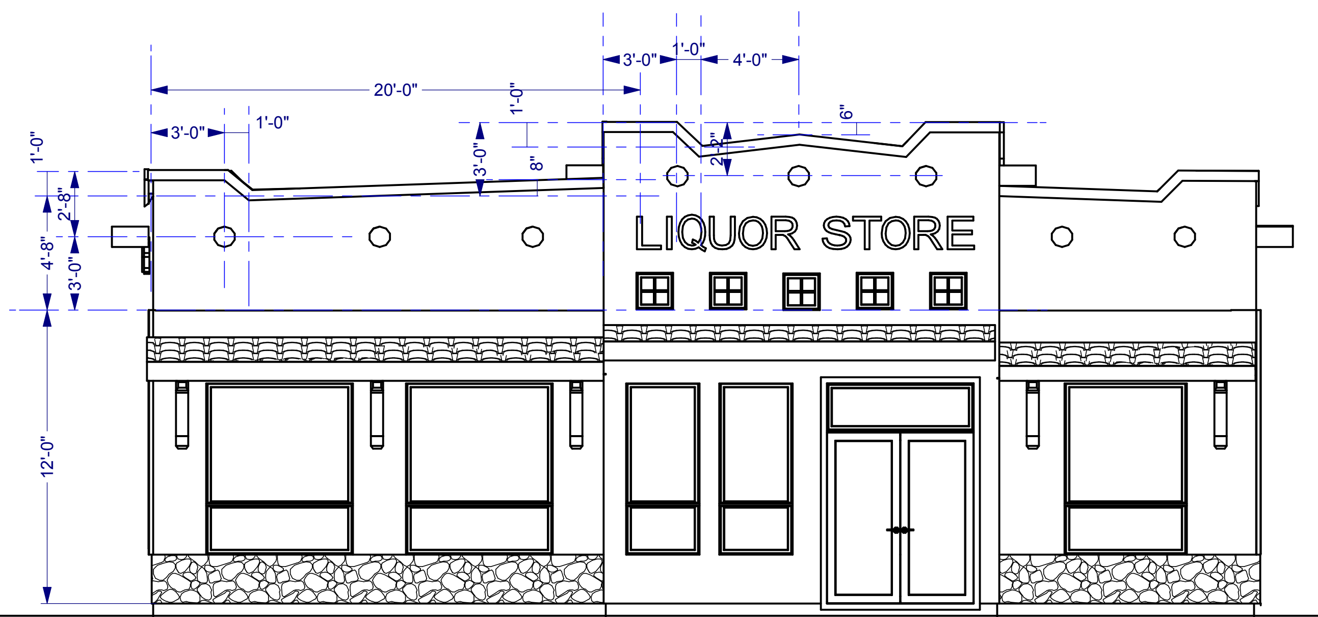
FRONT RIGHT RAISED PARAPET ELEVATION Scale: 1/4" = 1' - 0"
