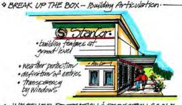
· WEATHER PROTECTION & PEDESTRON SCALE
